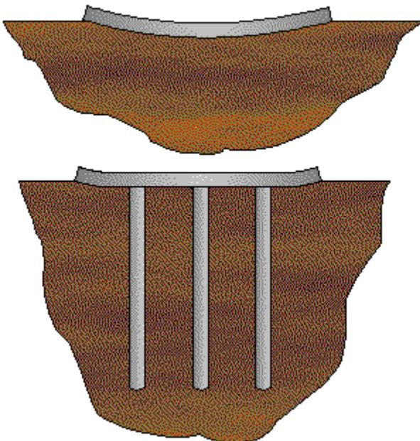
Settlement reducing piles are usually incorporated beneath the central part of a raft foundation in order to reduce differential settlement to an acceptable level. Such piles act to reinforce the soil beneath the raft and help to prevent dishing of the raft in the centre.
