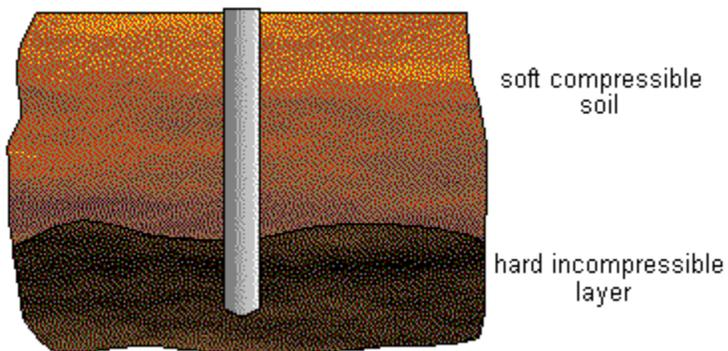
End bearing piles are those which terminate in hard, relatively impenetrable material such as rock or very dense sand and gravel. They derive most of their carrying capacity from the resistance of the stratum at the toe of the pile.
