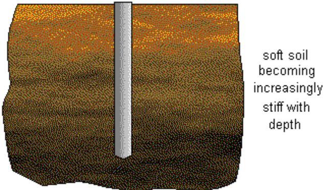
Friction piles obtain a greater part of their carrying capacity by skin friction or [adhesion](#). This tends to occur when piles do not reach an impenetrable stratum but are driven for some distance into a penetrable soil. Their carrying capacity is derived partly from end bearing and partly from skin friction between the embedded surface of the soil and the surrounding soil.
