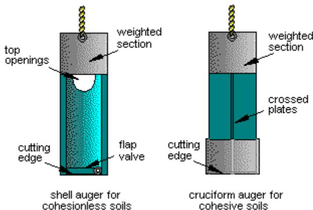
These tend to be 600mm or less in diameter and are usually constructed by using a tripod rig. The equipment consists of a tripod, a winch and a cable operating a variety of tools. The basic tools are shown in this diagram.
